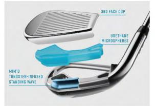
Because the urethane is lighter than the steel area it supplants, it had to be balanced with a piece of MIM'd tungsten in order to achieve the proper weight and CG location necessary to the iron's performance goals. MIM stands for "metal-injected molding," a process that allows us to form highly dense alloys into sophisticated shapes.
